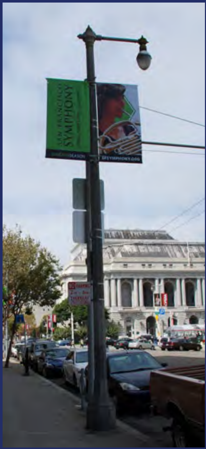
Aggregate concrete streetlight post with right angle pendant at Grove St
